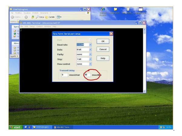
This is required because the standard serial port of the Arduino firmware doesn't use any handshaking control.
