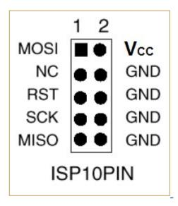
So you must consider this when connecting the USBasp to the 6 pins ICSP port (J3) on the Z80-MBC2 (see the schematic):
