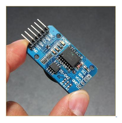
This cheap modules have a trickle charging circuit that may cause the "explosion" of the battery if you use a standard CR2032 cell. More, it can damage also a rechargeable LIR2032 cell. For more information and how to fix it see *here*.
