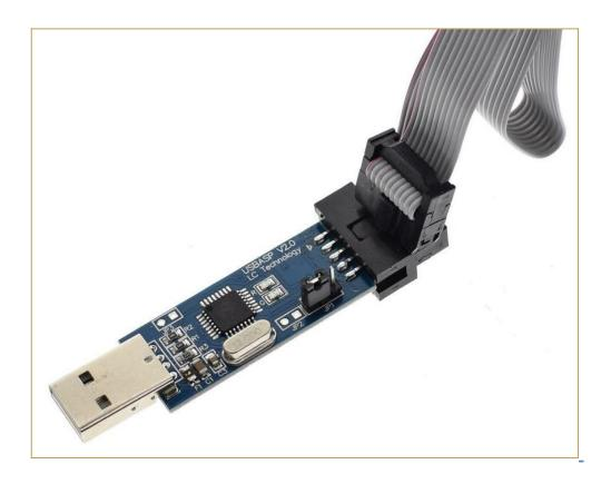
The USBasp is also capable to give the power to the "target" using the VCC pin, but remember to **check that the JP1 jumper is set to provide 5V to the target** (as shown in the photo).
