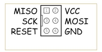
To avoid problems I suggest to use as GND pin 10 of the USBasp connector, and connect the other pins (VCC, MISO, MOSI,SCK, RST) accordingly. An handy way to connect the USBasp to the 6 pin ICSP port (J3) of the Z80-MBC2 *could be* to use a commonly available "10pin to 6pin" adapter like this:
