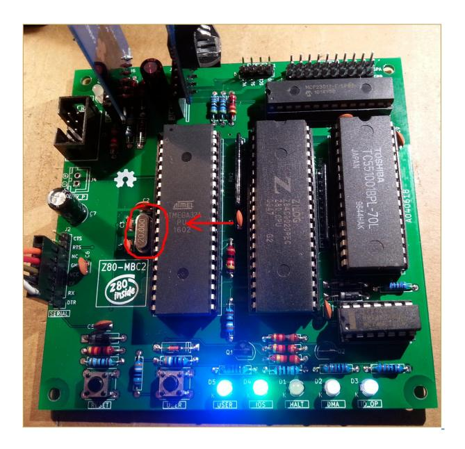
You don't need others HW changes, just use a 20MHz quartz instead of a 16MHz one. The Z80 clock speed will be at 10MHz.
